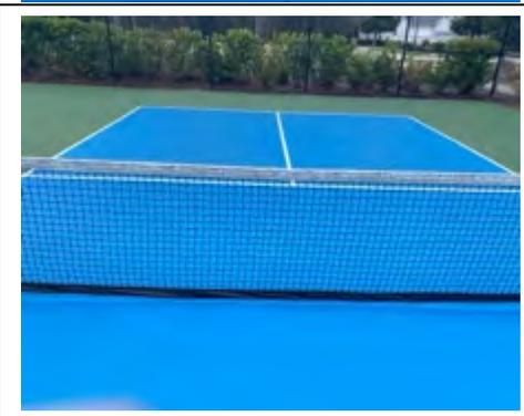
Multiple cracks throughout the pickleball court need patching. Additionally, the court requires cleaning and resurfacing with paint. I also recommend cleaning the tops of the nets and replacing the cracked composite benchboards located just outside the pickleball court.
